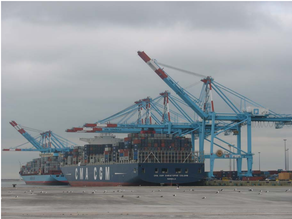
The 14,000 TEU CMA-CGM Christophe Colomb at APM Terminals Zeebrugge on October 5 th -6 th where 139.8 moves per hour berth productivity were registered.
