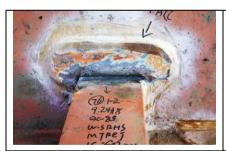
VT inspection after crack removed by grinding
