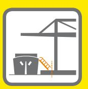
Gangway accommodation should be safely accessible from the quay and provided with a net unless the gangway is "closed".
