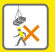
Never walk under a load. Please note when working with onboard crane where Ship to shore crane is located or moves.
