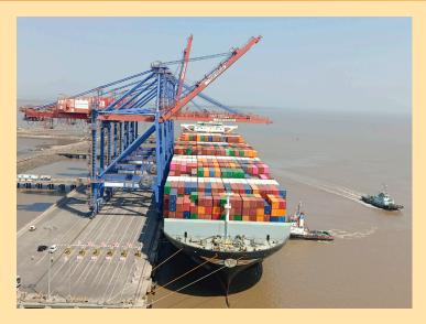
The port welcomed the largest container vessel ever at the port in February 2022. MV Express Athens from Hapag Lloyd is deployed in the TP1 INDAMEX service that caters to the USEC trade. EXPRESS ATHENS has a length overall (LOA) 349 m, beam 49 m, gross tonnage of 113973 and dead weight of 122959 was built in 2011 and can carry approx. 10114 TEU. The vessel came from Charleston terminal [US] and sailed to the Port Muhammad Bin Qasim [Pakistan].
