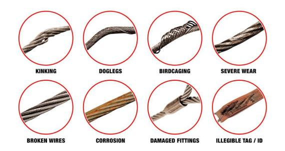
Any lifting tackle with visible mark of corrosion, crack, damage or made without proper heat treatment, **material should not be used**.
